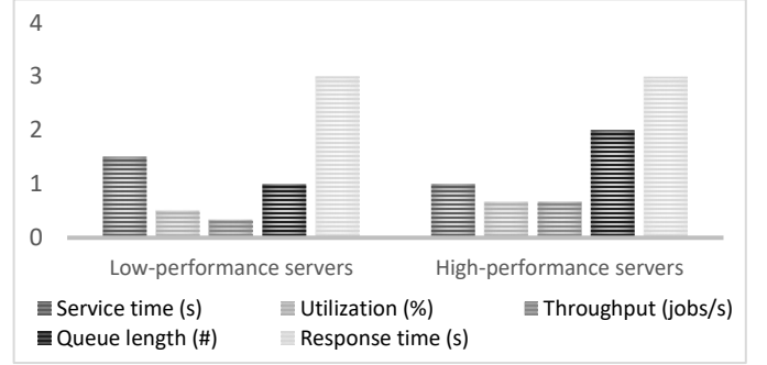
Figure 9. Mean values of important parameters of a heterogeneous datacenter with the pure-stochastic scheduler.
